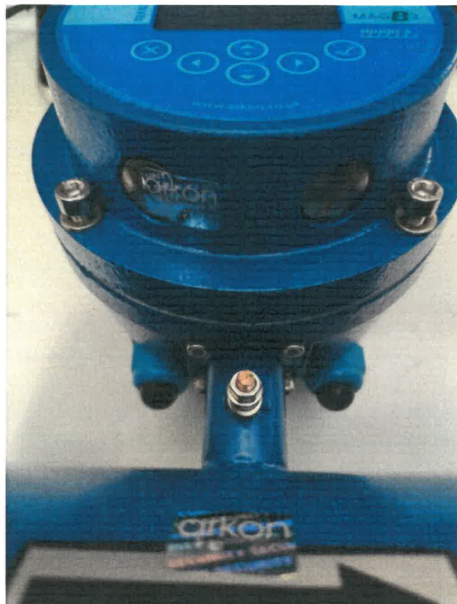
Figure 2: The water meter type MAGB2 – the screw covering the USB:
